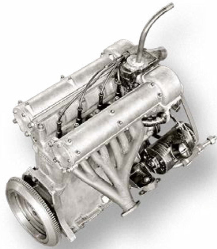
RS-Motor 1951, 4-Ventiler, 2 oben- liegende Nockenwellen (dohc)
